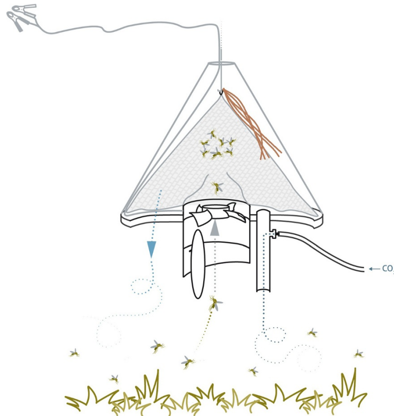
Figure 1 Cross-sectional schematic view of the Suna trap. When connected to a power supply the ventilator rotates and generates airflow under the cover of the trap. The air moves around an odour-bait (here shown as brown strips of nylon), which is suspended inside the trap between the catch bag and plastic trap cover. The air becomes saturated with odour that is attractive to mosquitoes. Air plumes leave the trap through holes in the trap base (blue arrow) and mosquitoes fly towards this attractive cloud of odour, as well as a plume of CO 2 , which is released through a pipe in the trap base. Mosquitoes that come close to the trap are sucked into the trap through the funnel and ventilator (grey arrow) and are captured in a bag where they die due to dehydration.
