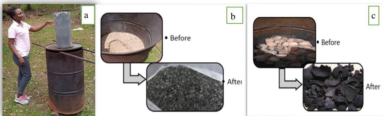
Plate 1: Setting of the TLUD (a), before and after pyrolysis of rice husks (b), coconut shells (c)
