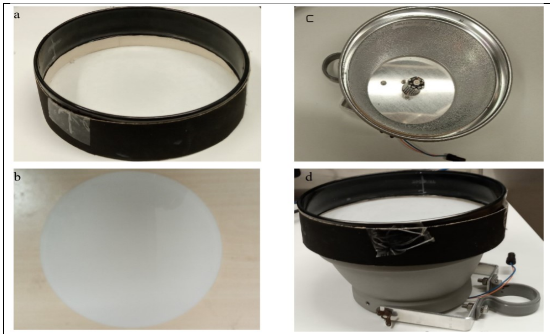
Figure 7: a =Petri dish, b=white glass, c = stand and bulb, d = complete water trap
