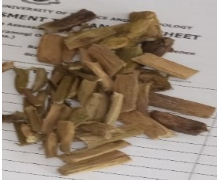
Figure 3. 1: Fully dried water hyacinth cubes and chops just before ball milling
