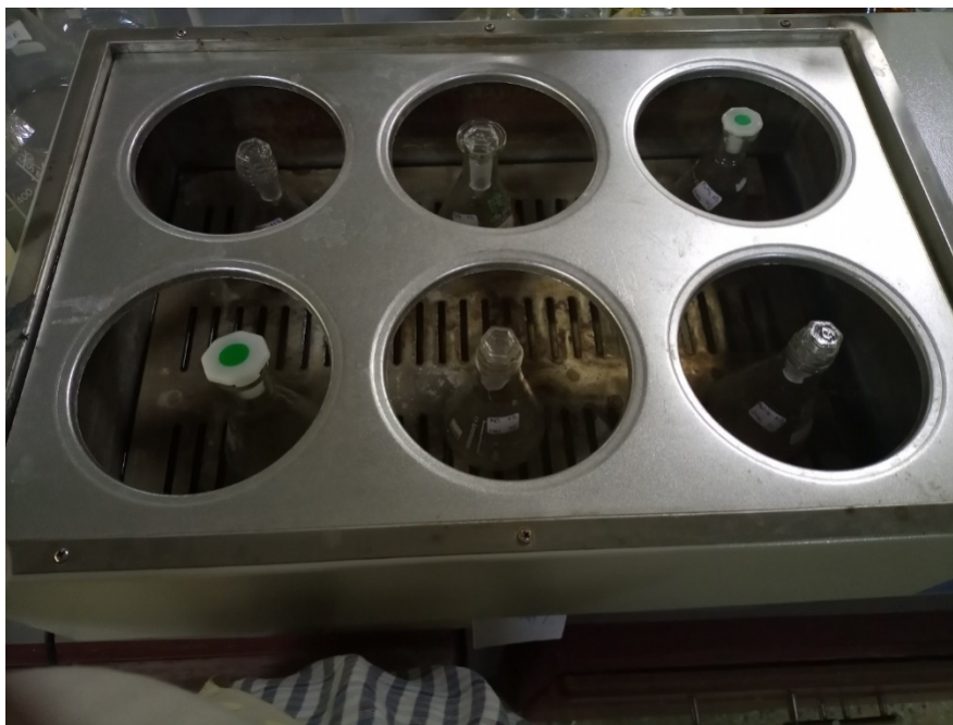
Figure 3. 5: Samples of extracted cellulose undergoing hydrolysis using same acid but of different concentrations being heated in a water bath at a uniform temperature
