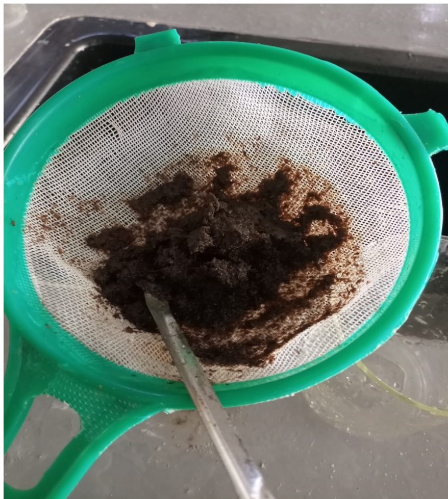
Figure 3. 3: Water hyacinth sediment product after alcohol pretreatment
