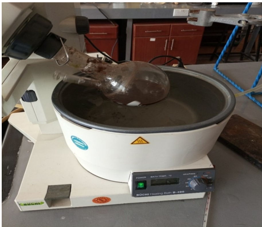
Figure 3. 2: Rotor-vap set up for the water hyacinth powder soaked in ethanol/toluene mixture being stirred continuously in an ever rotating round bottomed flask while being heated in the rotor bath
