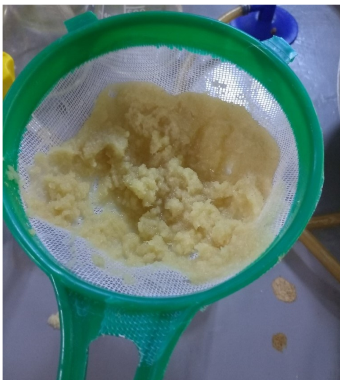
Figure 3. 4: The final product of the extracted CNCs from water hyacinth
