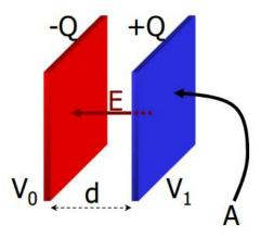
Show that the Capacitance of a parallel plate capacitor of plate areas A and separation distance
