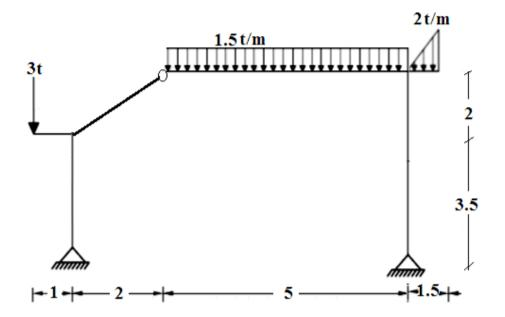
c, Draw the normal force, shear force and bending moment diagrams due to the applied load for the given cantilever in the Figure next. ? (5 Marks).
