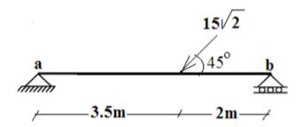
c. For simple beam (a-b) presented in Figure next, calculate the reactions at the two supports under the applied load? (8 Marks)
