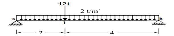
c. Draw the shear force and bending moment diagram due to the applied load for the given simple beam in the Figure next. ? (5 Marks).
