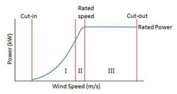
The power curve of a wind turbine indicates power output as a function of wind velocity at a hub height as shown in figure above. The curve shows the steady idealized characteristic.
