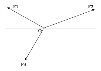
Given that F1 = 40N, F2 = 70N, F3 = 150N,  $= 28^{\circ}$ ,  $= 102^{\circ}$  and  $= 110^{\circ}$ , determine the magnitude and direction of the resultant force. (5 marks)
