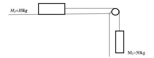
Determine the common acceleration of the masses and the tension in the string. (4 marks)
