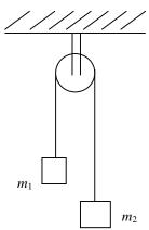
Show that the magnitude of the acceleration of the system a, and the tension T in the cord are given by:
