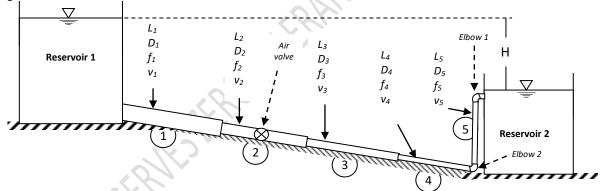
Using appropriate formulae identify all major and minor losses that would occur in the system. Additionally, Given H as the total head between Reservoir 1 and 2, express the available Head that the system will have to ensure water is delivered to Reservoir 2 (20 Marks)
