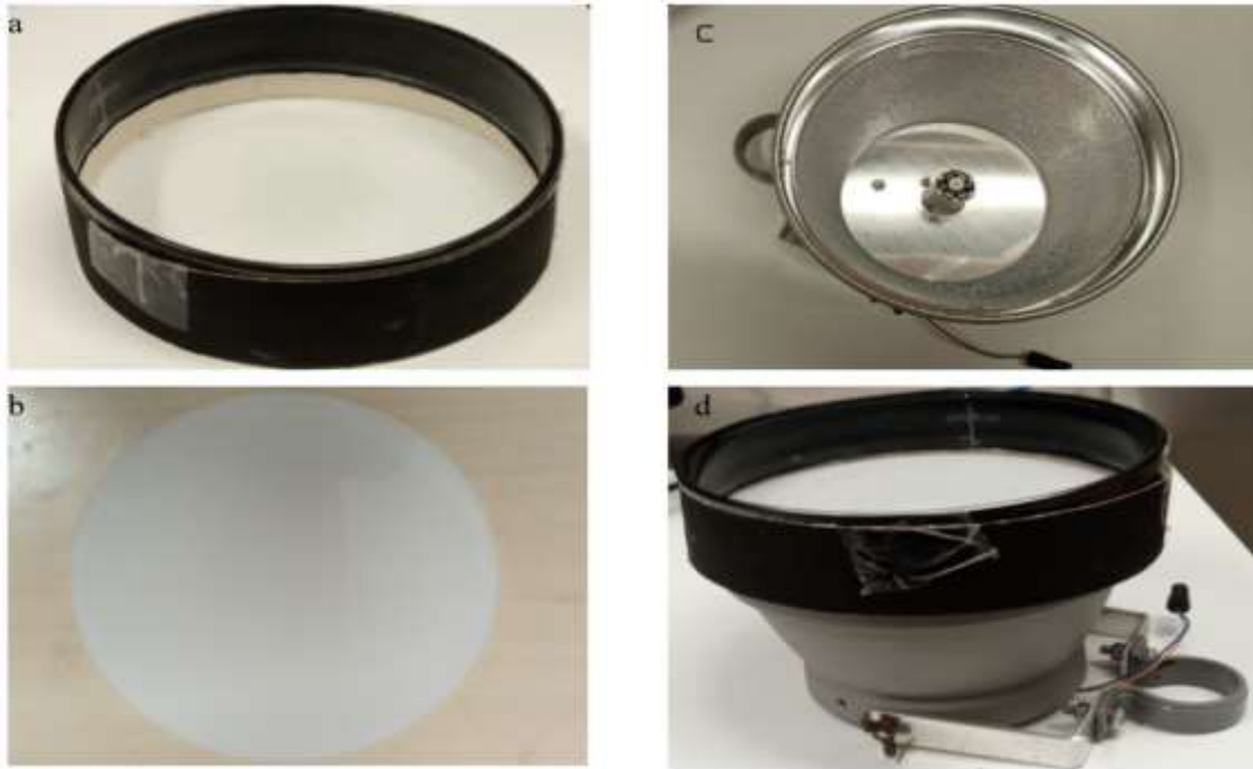
Fig 3a: Petri dish, b: light diffusing white glass, c: stand and bulb, d: complete water trap
