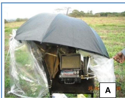
Figure 2A: Makeshift tent for pump when there was drizzle in the field.
