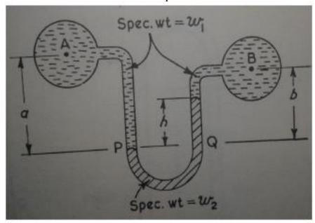
Calculate the difference in pressure if a=1.7m, b=0.95m and h=0.8m. Take the liquid at A and B to be water ( $w_i=9.81 \times 103$ N/m<sup>3</sup>) and specific weight of Mercury is 13.6 times that of water.
