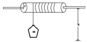
The windlass is a cylinder with a radius of 0.2 m and a momentum of inertia of 0.2 kgm<sup>2</sup>. If the bucket is released from rest, what is its speed just before it hits the water 10 m below (assume there is no friction or air resistance.) (3marks)
