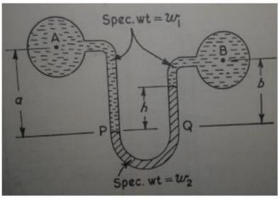
Calculate the difference in pressure if a=1.7m, b=0.95m and h=0.8m. Take the liquid at A and B to be water ( $w_i=9.81 \times 103$ N/m<sup>3</sup>) and specific weight of Mercury is 13.6 times that of water. (14 Marks)
