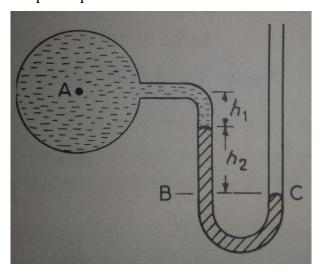
If the specific weight of Mercury is 13.6 times that of water at atmospheric pressure (101.3KN/m), what is the absolute pressure at A when  $h_1=15cm$ ;  $h_2=30cm$ ; Specific weight of water =  $9.81x \cdot 10^3 \text{N/m}^3$
