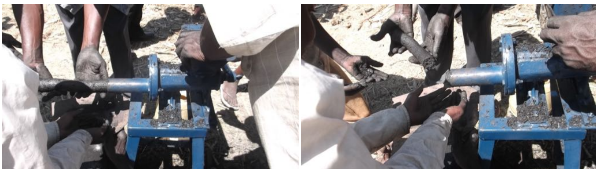
Plate 7: Damp briquette extrusion.
