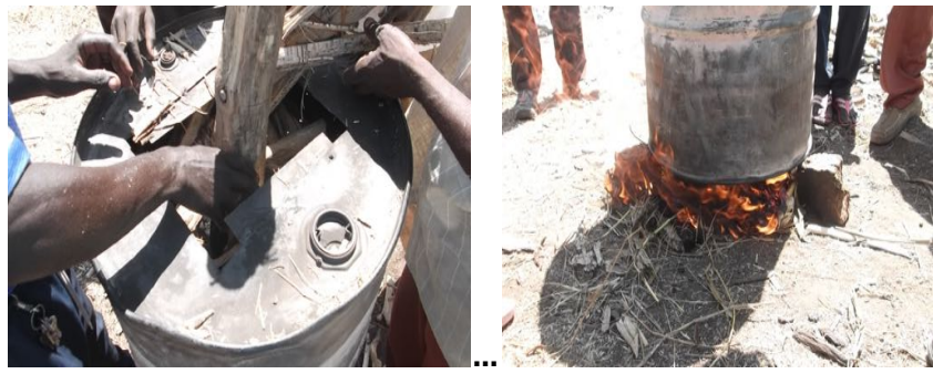
Plate 3: a) Distribute material evenly around centered log, b) Ignite base.
