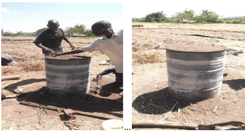
Plate 5: a) Drum removed from stove. b) Sealed to burn anaerobically.
