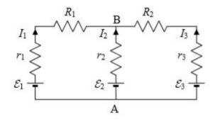
Take  $\mathcal{E}_1 = 6 \text{ V}, r_1 = 1\Omega, \mathcal{E}_2 = 10 \text{ V}, r_2 = 2\Omega, \mathcal{E}_3 = 12 \text{ V}, r_3 = 3\Omega \text{ and } R_1 = R_2 = 20\Omega$  [6marks]
