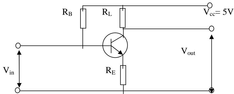
Note:  $R_E = 1.25 \text{ k}\Omega$ ,  $R_L = 5 \text{ k}\Omega$ , and  $R_B = 530 \text{ k}\Omega$
