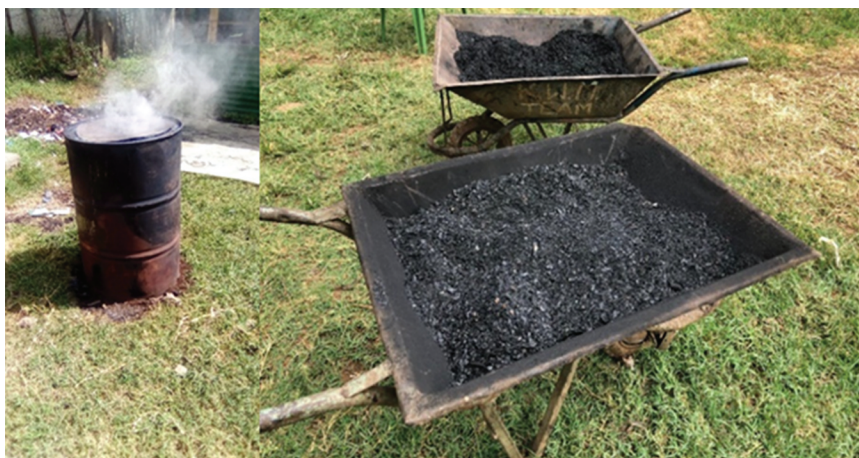
Figure 1. Updraft carbon kiln and carbonized market waste.
