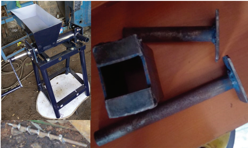
Figure 2. Manual screw press and its overhanging screw shaft (left) and ram-piston press (right).
