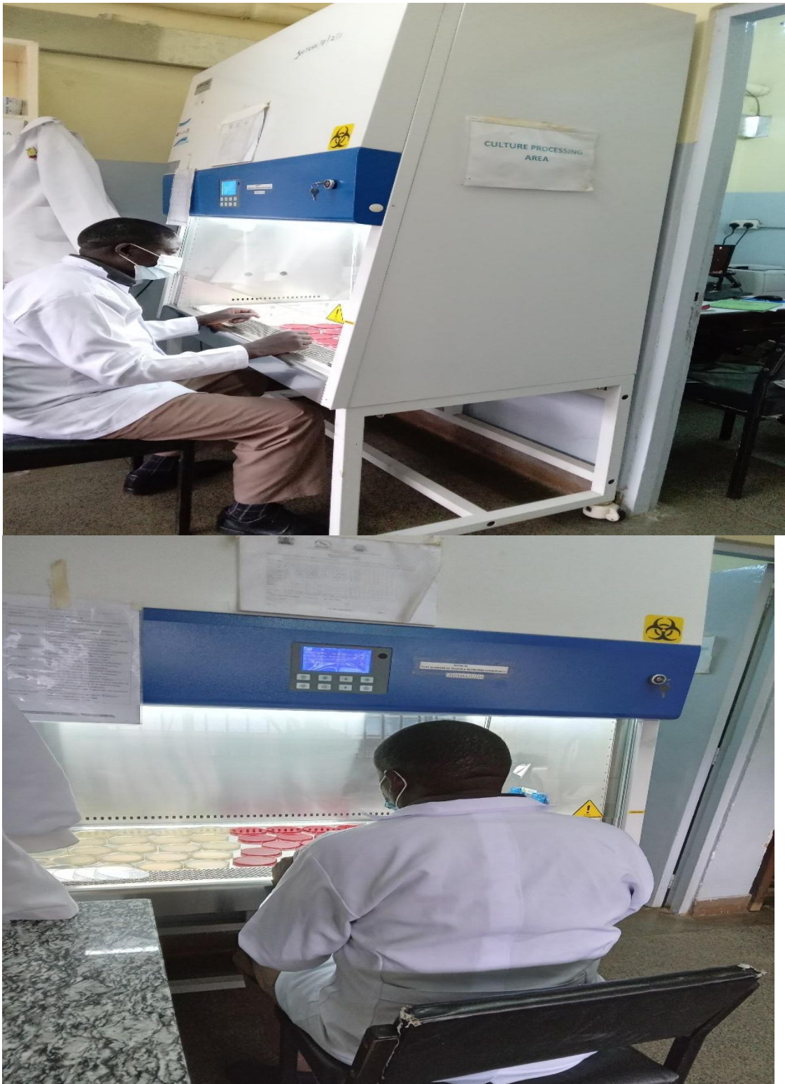
The above photo shows a technologist in the process of media preparation inside a biosafety cabinet
