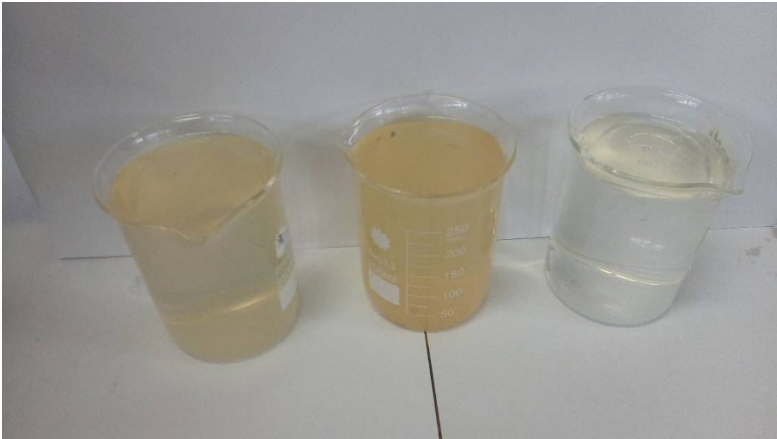
Figure 3: Changes in turbidity as the water passes through the different stages
